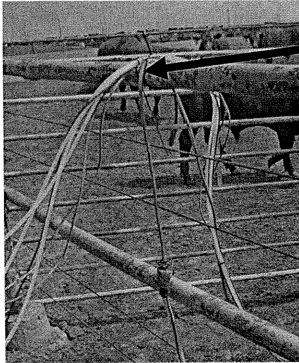
Figure 3. Location of gas sampling port for semi-continuous measurements of ambient air H 2 S concentrations at Feedyard C.
