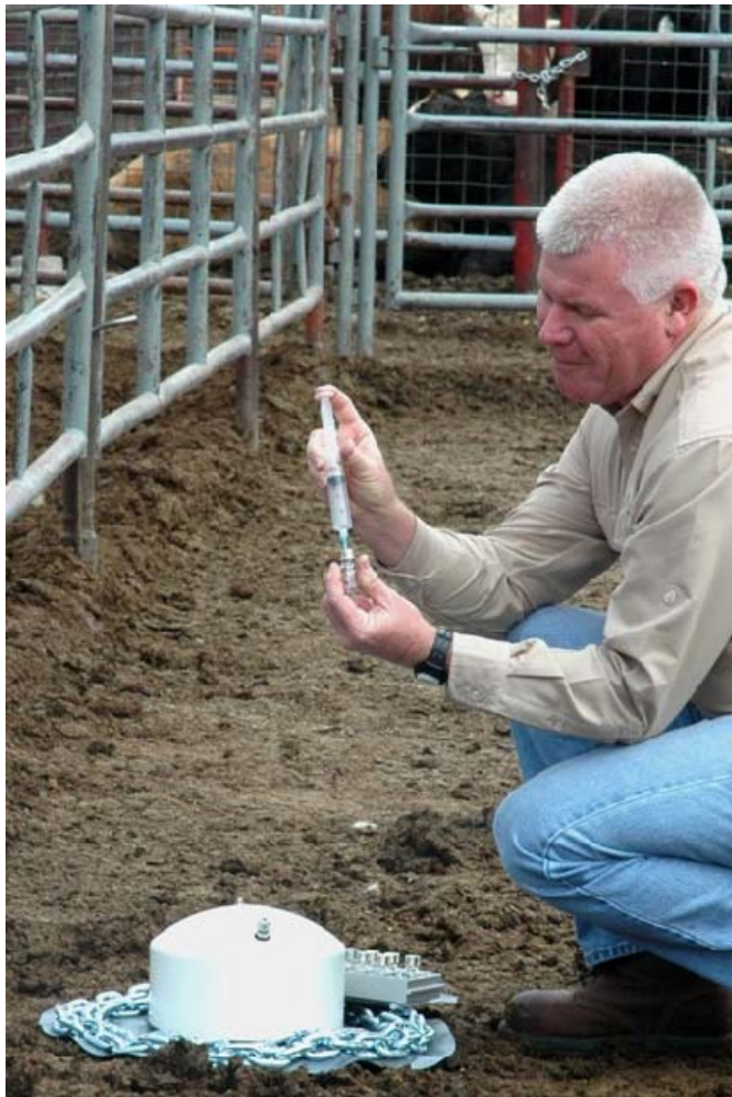
Figure 3. Injecting a gas sample collected from the NFF-NSS chamber into an evacuated vial.
